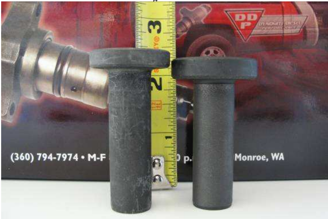
12 valve lifter on left and 24 valve on right
