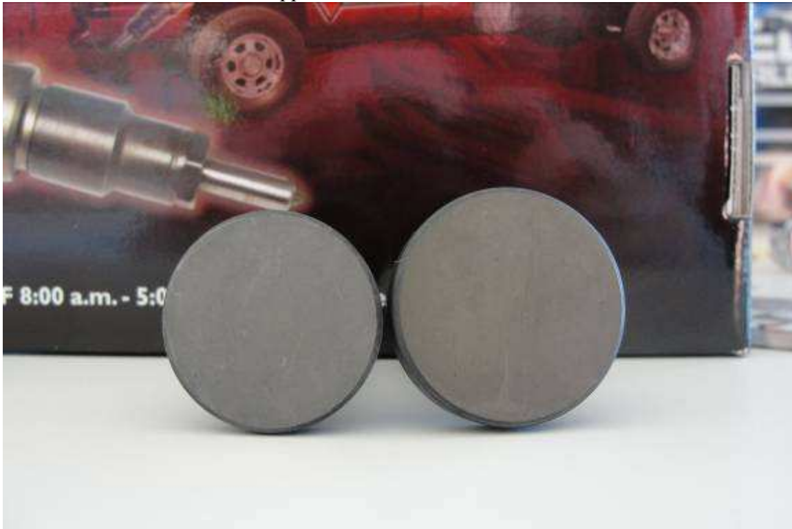
12 valve lifter on left and 24 valve on right
