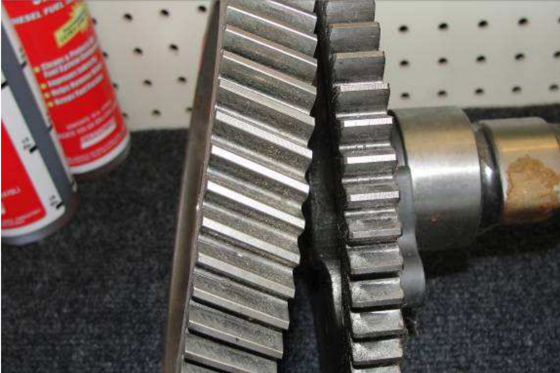
Common Rail gear on right and helical gear from 12v and 24v VP44 engines on left
